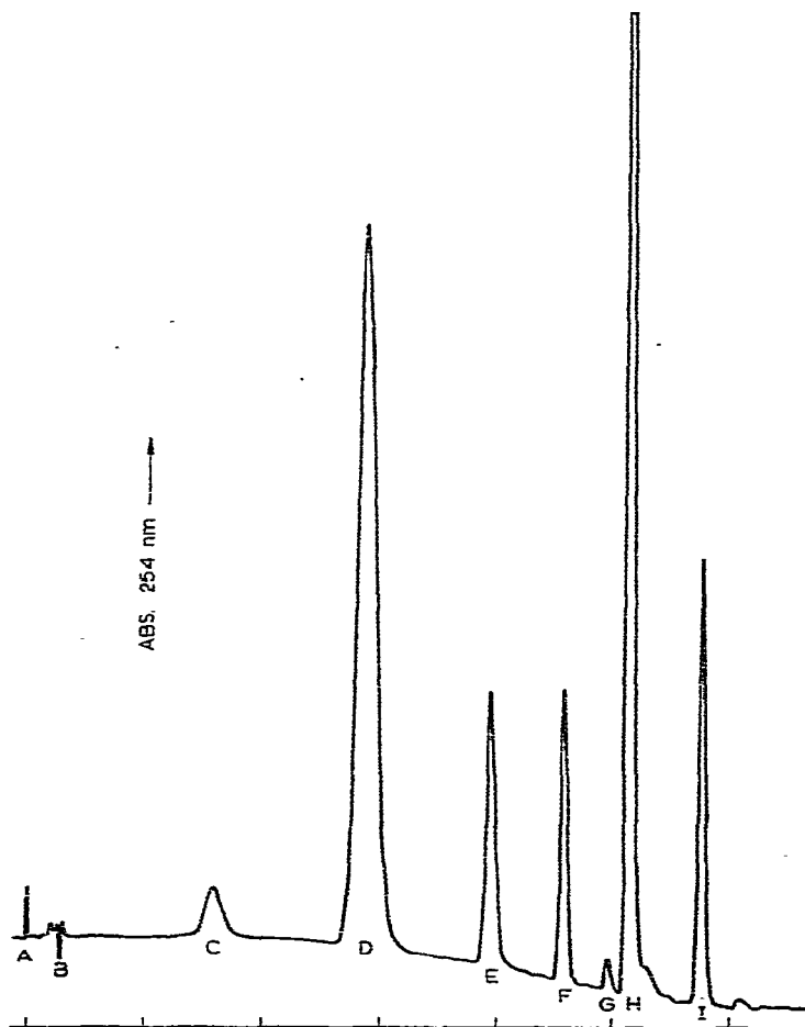
Fig. 1. Resolution of selected ureas. A = injection point; B = solvent front; C = 1,1-dimethyl-3-(1,1,1-trifluoro- o -tolyl)urea; D = 1,1-dimethyl-3-(1,1,1-trifluoro- m -tolyl)urea; E = 1,1-dimethyl-5-(1,1,1-trifluoro- m -tolyl)urea; F = 1,3-bis(1,1,1-trifluoro- o -tolyl)urea; G = impurity related to H; H = 1,3-bis(1,1,1-trifluoro- m -tolyl)urea; I = dimethylphthalate internal standard. Concentration adjusted to 8 mg/ml for sample components and 2 mg/ml internal standard. See text for experimental conditions. R_f /sec: C = 390; D = 690; E = 960; F = 1110; H = 1245; I = 1395.
